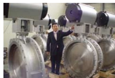
POSCO FINEX Main Facility CONTROL VALVE 1000A
