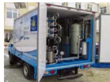
Mobile Water Purification System
